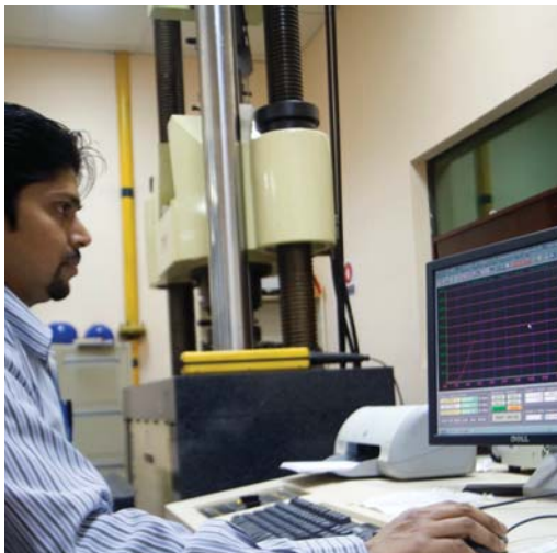
Universal Tensile Testing Machine (UTS) (1000 KN Computerised)
