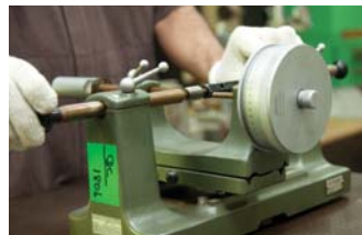
Gauges Calibration (Floating Carriage Micrometer)
