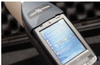
Alloy Analyzer (USA) (Positive material identification)
