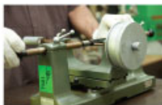
Gauges Calibration (Floating Carriage Micrometer)
